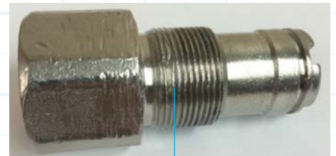
Damage to threads on SDX III Nozzle
